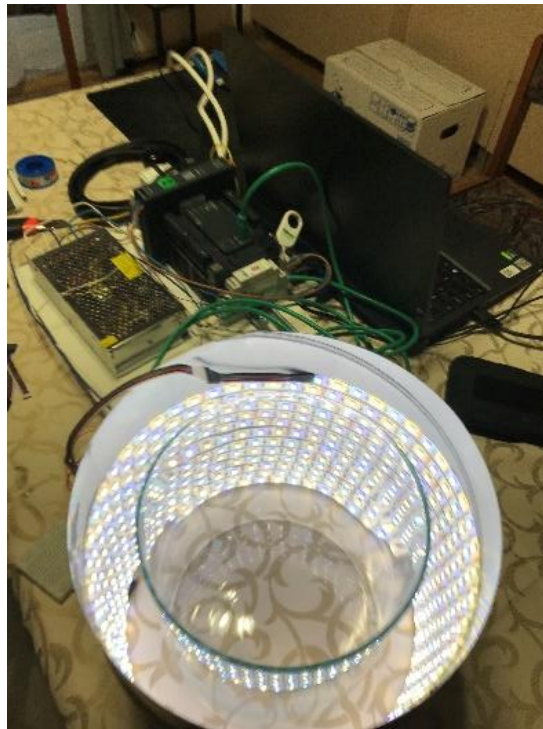
Fig. 2. Automation of the lighting control system for phytotrophic farms
