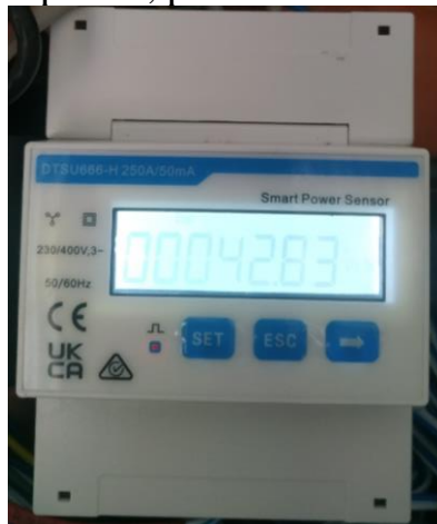
Fig. 1. Intelligent power meter DTSU666-H 250 A / 50 mA
