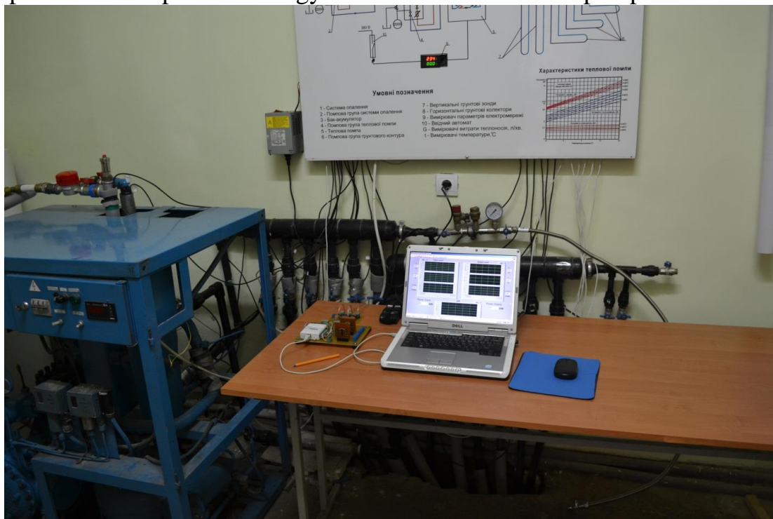
Fig. 2. Laboratory model for the study of heat pump operating parameters such as "ground-water".
